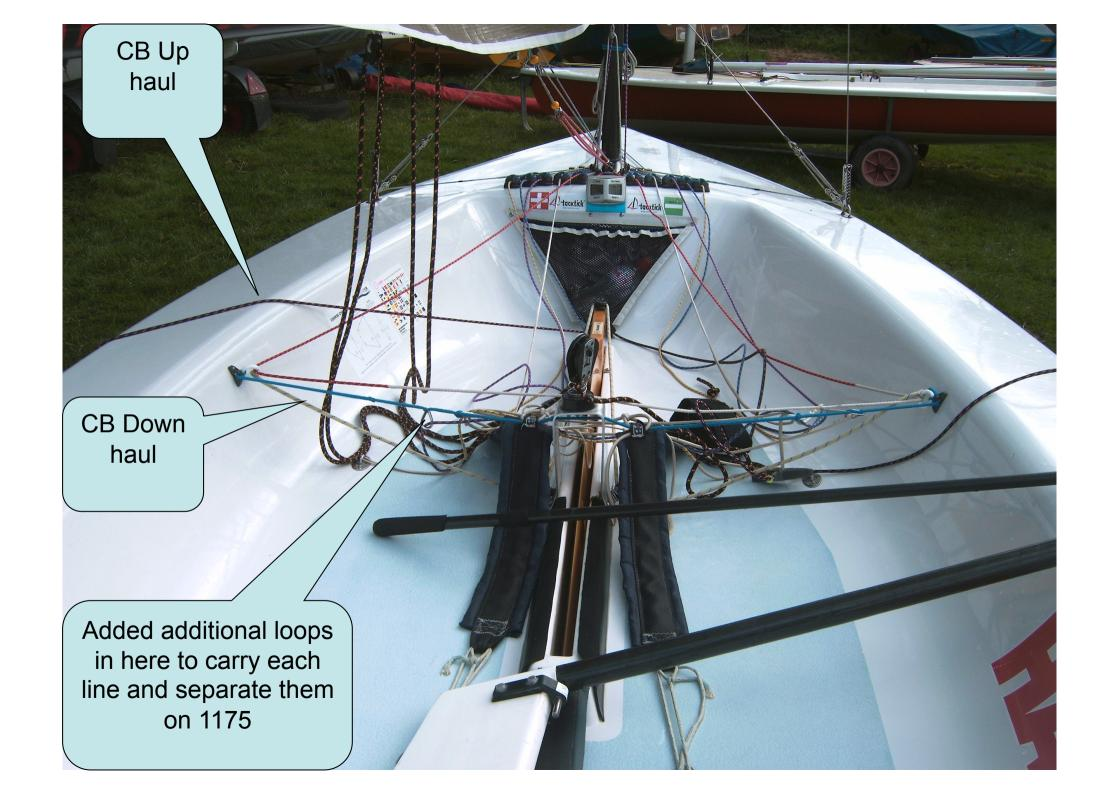
Centre Board has Up haul and down haul, no elastic.
