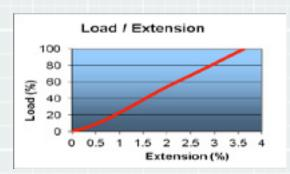
Typical working elongation (for bedded in rope)
