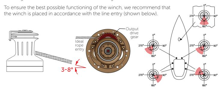
Be also aware that the self-tailing arm is positioned correctly. We recommend to have the self-tailing arm positioned within the shaded area (shown above). On this model the self-tailing arm is fixed, making it very important to establish the proper location of the holes prior to drilling these in the deck.
