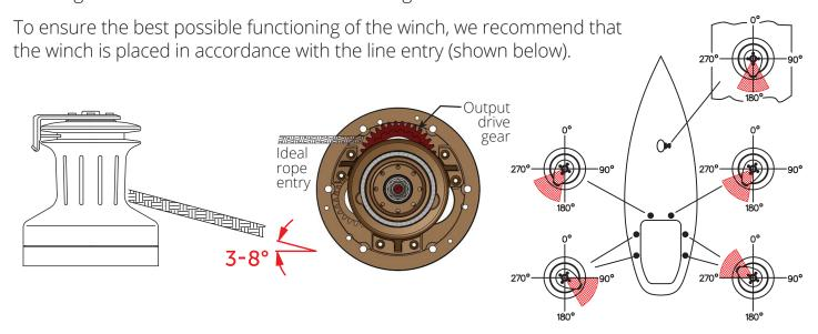
Be also aware that the self-tailing arm is positioned correctly. We recommend to have the self-tailing arm positioned within the shaded area (shown above). On this model the self-tailing arm can be placed in several different positions after having installed the winch.
