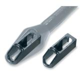
It is essential to lock the line securely for the compensator to work properly. Forsheda mooring compensators are equipped with locking elements at both ends which are vulcanized into the compensator. The lock elements, which are injection-moulded and made of polyamide 6 (nylon). lock the line securely without causing wear.
