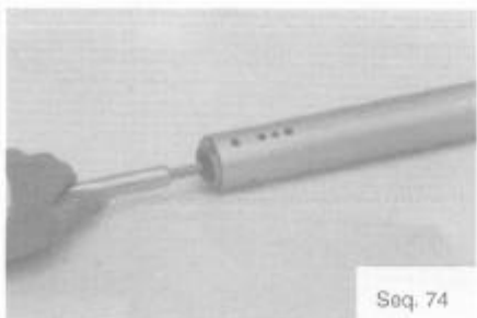
Le câble est centré. Stay is centered in extrusion.
