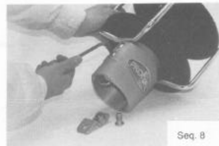
Seq. 8 Démontez les deux vis de lattes. Unfit both link plates set screws.
