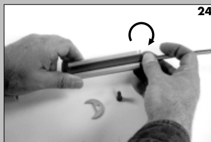
Tournez le palier de 1/4 de tour Turn the bearing by 1/4 turn
