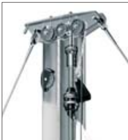
Seldén in-mast furling system: Geared line driver winch, tensioned luff extrusion, assymetrical located sail slot and the patented load distributor of the halyard swivel. All to make furling an easy and fast operation.
