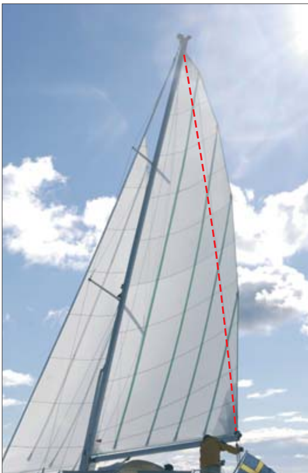
Seldén in-mast furling system: Geared line driver winch, tensioned luff extrusion, assymetrical located sail slot and the patented load distributor of the halyard swivel. All to make furling an easy and fast operation.
