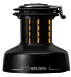
The drums we are using for our new manual and electric winches are forged and machined hard anodised aluminium with vertical ribs located in an asymmetric pattern. Any line under load will become slightly dented where it rests over a rib and if all ribs were located symmetrically, all dents would simultaneously jump to the next rib when releasing the line. And the next one, and the next one...
