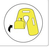
4. Remove one of the Lume-On™ stickers from the packaging, remove the backing paper. Stick the Lume-On™ to the bladder in a position:
