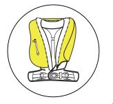
**2.** Lay the inflatable bladder on a table, as flat as possible.
